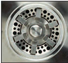
Dual stages: primary axial and secondary radial
