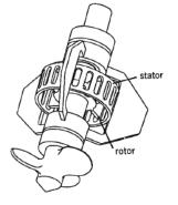
A rotor/stator mixer is a common high-shear mixer used in sanitary processing. The rotor is a rotating impeller that rotates at a high speed to move the product from the inside to the outside through the stator. The stator is the stationary cage or shell with very close clearance to the rotor. A high-shear area is formed as the product is forced through the small clearances between the rotor and stator. This action reduces particle size and increases surface area for better
