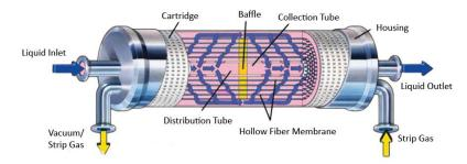
Applying a higher pressure to the liquid stream relative to the gas stream creates the driving force for dissolved gas in the liquid to pass through the pores in the membrane. The gas is then carried away by the vacuum pump or strip gas. Water does not enter the micropores but are held back due to the hydrophobic nature of the polymer and the surface tension across the membrane.
