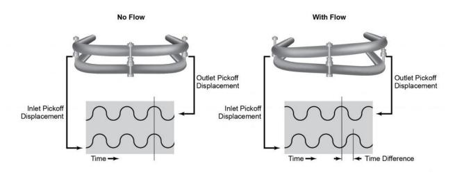
This effect can be experienced when riding a merry-go-round – when moving toward the center, a person will "lean into" the rotation to maintain balance. Most flowmeters have a split coil design. During operation, a drive coil stimulates the tubes to oscillate in opposition (sine waves). A sensor measures the time delay between the two sine waves (Delta T) which is directly proportional to mass flow rate.
