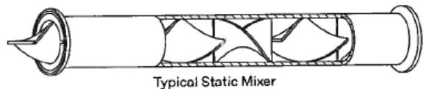
Static mixers are not commonly found in sanitary processing but offer a low-energy mixing alternative for liquids that are easily miscible. It is used for continuous processing applications in which a tube or housing is fitted with baffles. The baffles may be constructed of stainless steel, Teflon®, PVC or other material.
