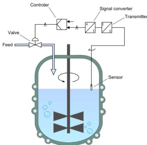
Let's look at a basic example. A level sensor measures the level in a tank and transmits a signal associated with the level reading to a controller. The controller compares the reading to a pre-determined value. If the level is low, the controller sends a signal to the valve on the feed line. The valve opens to add product to the tank and bring the level back to the correct position.
