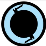
Concentric – used for most applications; the shaft is mounted in the center of the heat transfer tube
