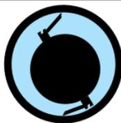
Eccentric – recommended for viscous and sticky products; design increases product mixing, eliminates mass rotation and reduces the mechanical heat load.
