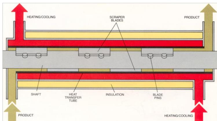
In operation, the product enters the cylinder at the bottom and flows upwards. The heating or cooling medium travels in a counter-current flow through a narrow annular channel. The rotating shaft has blades which continuously scrape product film from the heat transfer tube wall, thereby enhancing heat transfer, and agitating the product to produce a homogenous mixture
