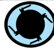
Oval – used for extremely viscous products; eliminates product channeling within the tube, reduces mechanical heat by a double cam action of the blades and balances the internal forces to prevent shaft deflection.
