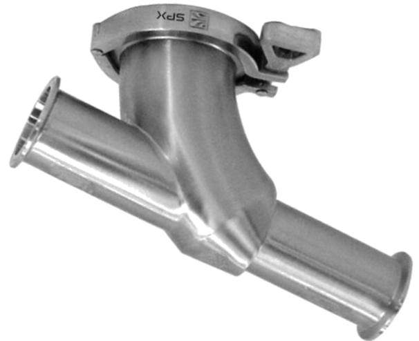
Thick, sticky products can also be problematic with ball check valves. In these cases, the ball can sometime stick in the Y branch and not properly reseal itself when flow stops. You can PIG your line through a ball check valve. Ball check valves have virtually no pressure drop.
