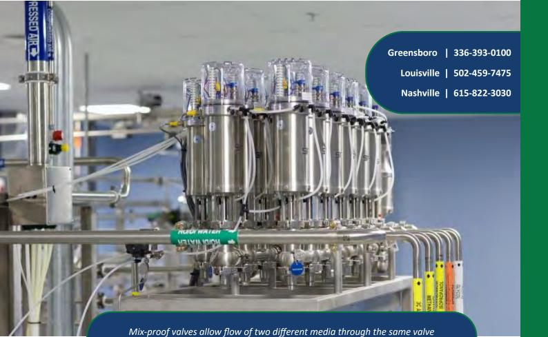
simultaneously without the potential for mixing.
