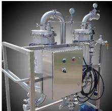
M.G. Newell engineers offered to design and fabricate a portable skid. The skid design included two Liqui-Cell<sup>®</sup> gas membrane contactors specifically sized for their desired capacity and pump size. The layout also included a UV sanitizer and instrumentation including a UL Certified<sup>®</sup> control panel. Our engineers ensured integration of the skid within their existing system of flow valves, analytical instrumentation, and tank level controls.
