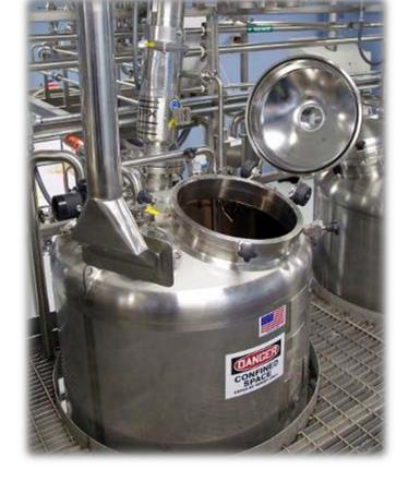
Single-wall or jacketed designs Fully customizable Standard bottom configurations—conical, dish, flat-sloped Standard top configurations—open, dome or bridge & cover Various agitation options available Electropolishing and passivation available
