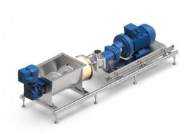
The M.G. Newell account manager thought that a **twin-screw pump** would be a good solution. He contacted the pump manufacturer who brought in a demo pump to try on the meat slurry. The twin screw pump was able to push the slurry through the 4" line and it was able to suck the slurry from the hopper. After the trial, the customer upsized to a 5" inlet on the pump to further improve the suction capabilities on this high-viscous slurry.
