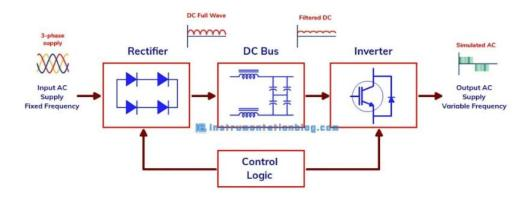
The **rectifier/converter** is the first of the three sections of a VFD's main power circuit, and first in terms of power flow. Incoming AC line voltage is rectified or converted to DC voltage in the converter section, which consists of diodes, silicon-controlled rectifiers (SCRs), or insulated gate bipolar transistors (IGBTs)
